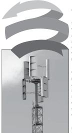
VBINE has developed the worlds first direct drive vertical axis wind turbine.
