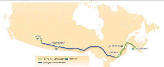
TransCanada officials were in Moosomin to provide an update on the Energy East pipeline proposal. Energy East would include a feeder pipe-line from Cromer, Manitoba to the Moosomin compressor station, and a tank farm at Moosomin to store crude oil production from the Bakken oilfield.
