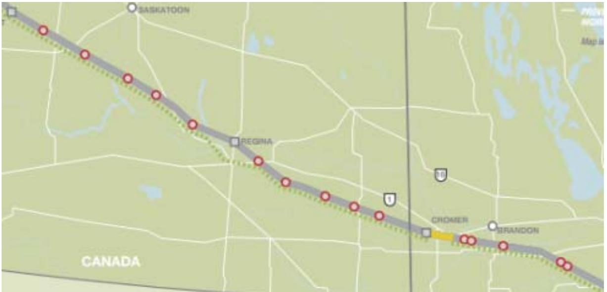
The Enbridge Line 3 route across Saskatchewan and Manitoba. A short section of Line 3 east of Cromer has been replaced already. The rest will be replaced as part of the new project.
