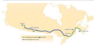
TransCanada officials were in Moosomin to provide an update on the Energy East pipeline proposal. Energy East would include a feeder pipeline from Cromer, Manitoba to the Moosomin compressor station, and a tank farm at Moosomin to store crude oil production from the Bakken
