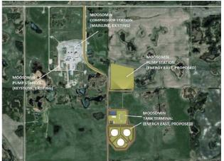
The proposed Energy East pipeline project would include a tank farm at the Moosomin compressor station and a feeder pipeline from Cromer to Moosomin.
